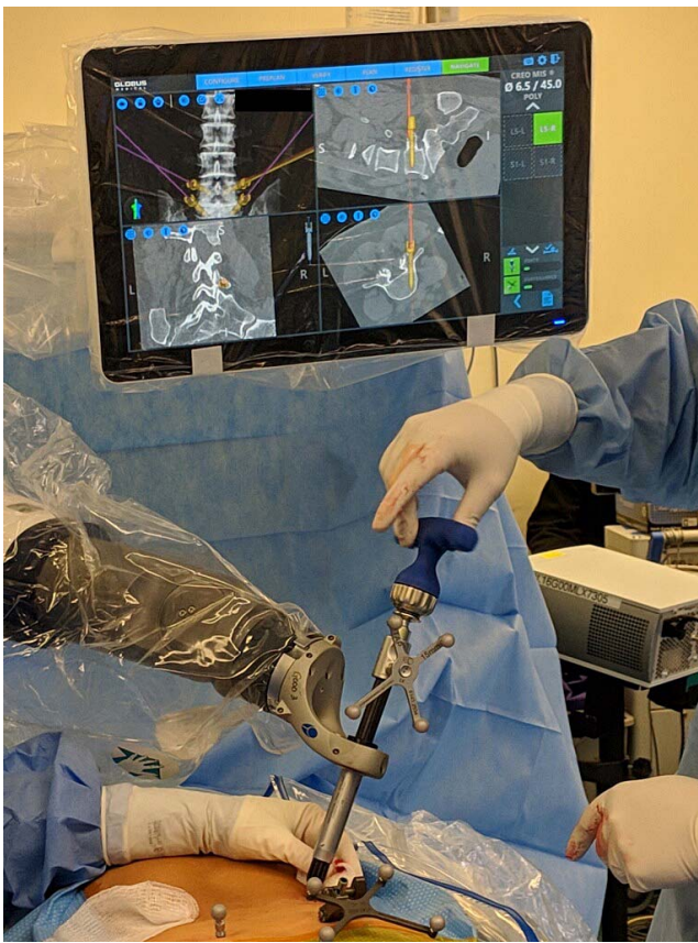
Figure 2. Intraoperative photo of screw insertion through the robotic arm. The screw is displayed overlying the CT on the display.
