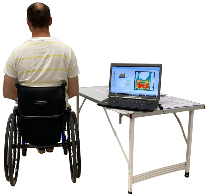
Figure 1. Measurement setup. Measurements were taken using a pressure mat (BodiTrak2, 16 \times 16 = 256 sensors) placed on the participants own seat cushion in their own wheelchair. Using the standard supplied FSA.1 software package, the following parameters were measured: maximum pressure (mm Hg), mean pressure (mm Hg), measurement area ( \text{cm}^2 ) as well as the coordinates of the center of pressure (cm).
