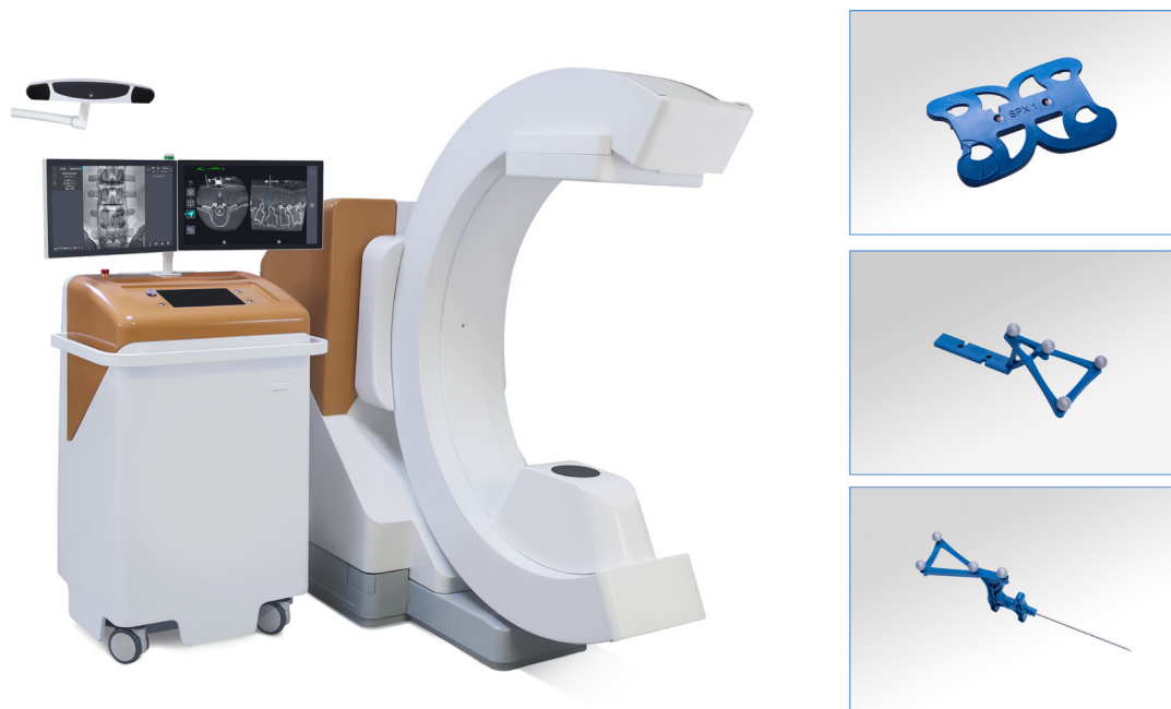
Figure 1. Depiction of the Surgivision surgical platform. Left: Unified platform composed of a C-arm, a navigation station, and an infrared camera. Right: Surgivision disposable instruments (from top to bottom): imaging phantom, patient tracker, and navigated trocar.
