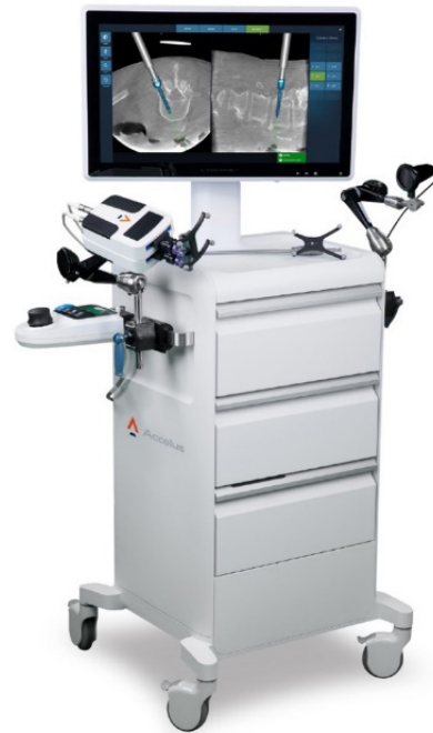
Figure 1. Accelus Robotic Navigation System including nearfield camera (200 g) and robotic arm (2.2 kg) affixed in the storage position to the display monitor and cart.
